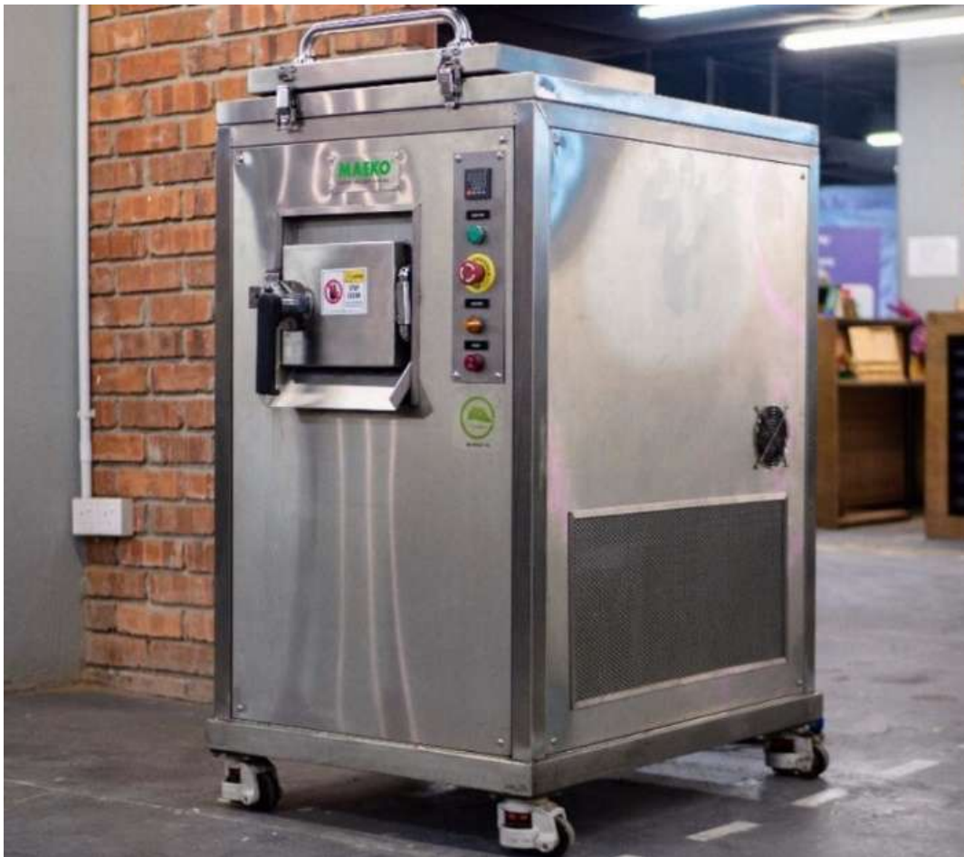
Figure 6.4.6 Maeko composter, which can produce compost in 24 hours.
