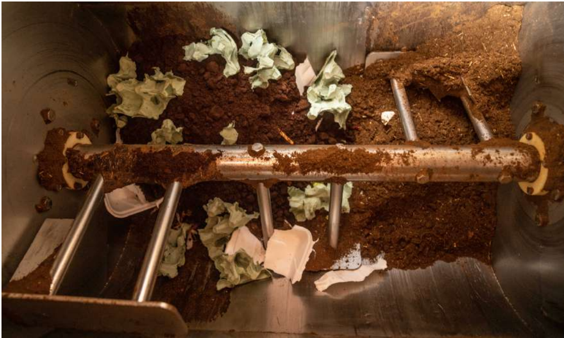
Figure 6.4.1 Interior of the aerobic composter being trialled on a pilot scale by Zero Waste Alliance Ireland, showing the rotating mixer which keeps the food waste aerated.
