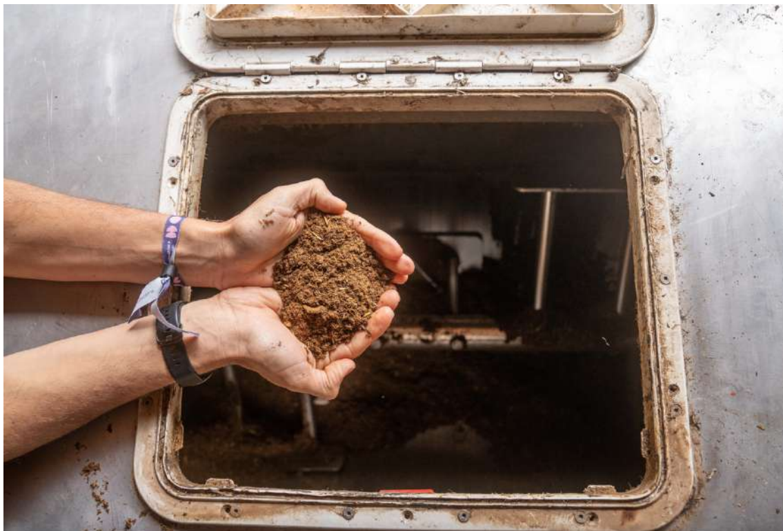
Figure 6.4.2 Sample of the compost produced by the Zero Waste Alliance Ireland composter; this machine, which incorporates a heating element, produces compost in 24 hours, utilising thermophilic micro-organisms.
